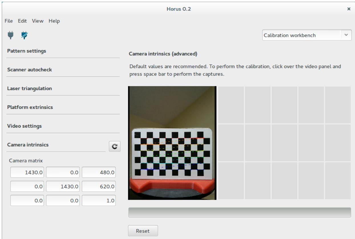
**Warning:** If camera intrinsics values are modified, laser and platform calibrations must be performed again.
