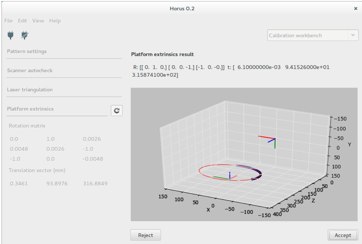
Once this process is completed, the scanner is calibrated.
