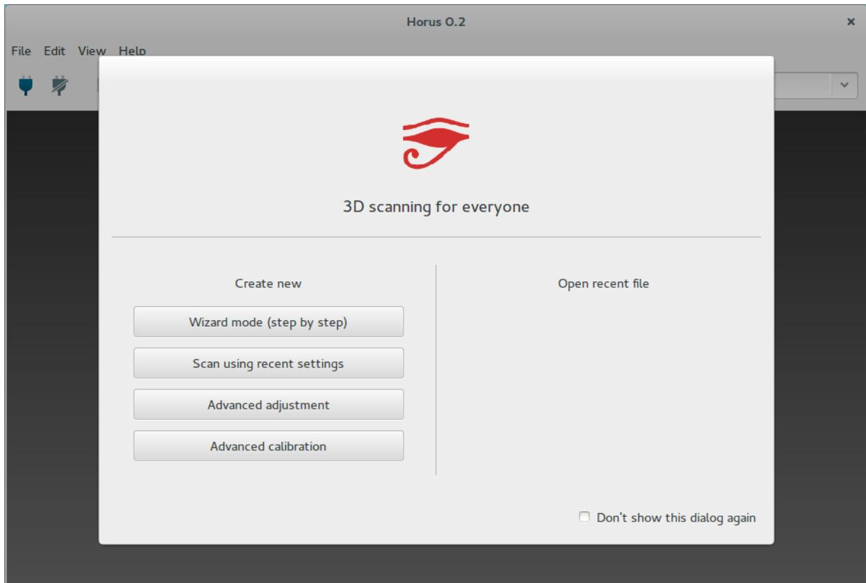
Pressing over **Wizard mode**, an interactive menu appears for configuring the scanner step by step.
