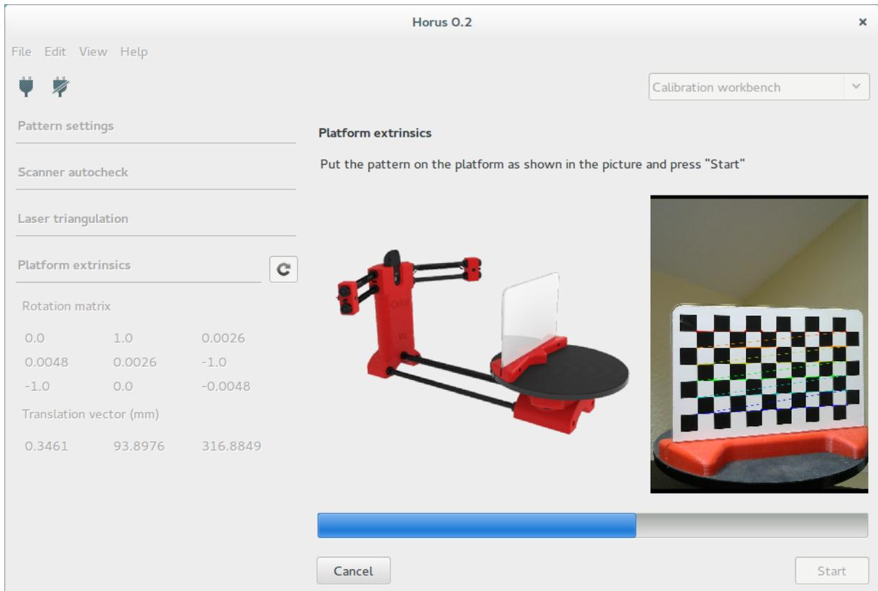
Finally the result is shown numerically and depicted in 3D. You can accept or reject the calibration result.
