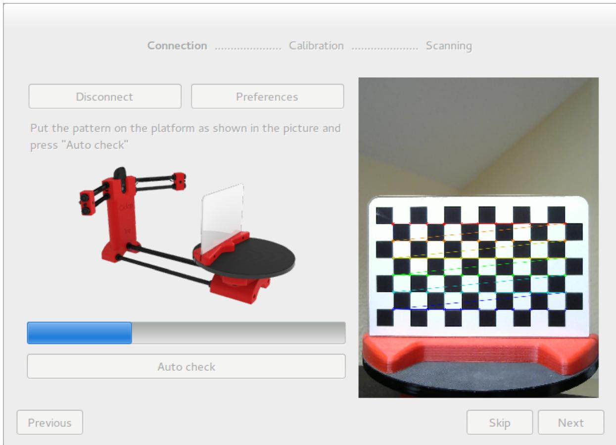
**Note:** The first time *Auto check* is pressed, a menu appears indicating if the lasers want to be aligned. This is for manually moving the orientation of the lasers until the emitted line is perpendicular to the platform. It requires an Allen wrench.
