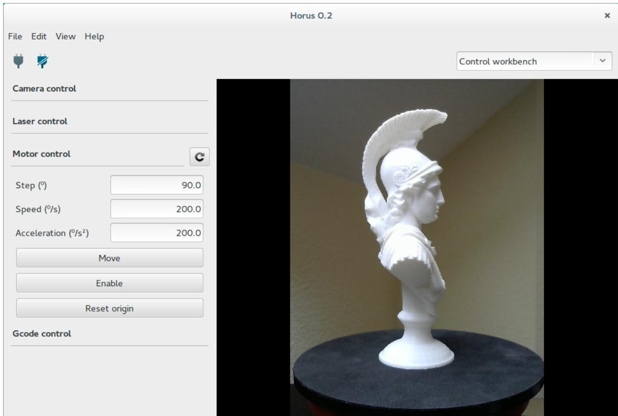
Also the motor can be enabled or disabled and the position stored inside the firmware reseted.
